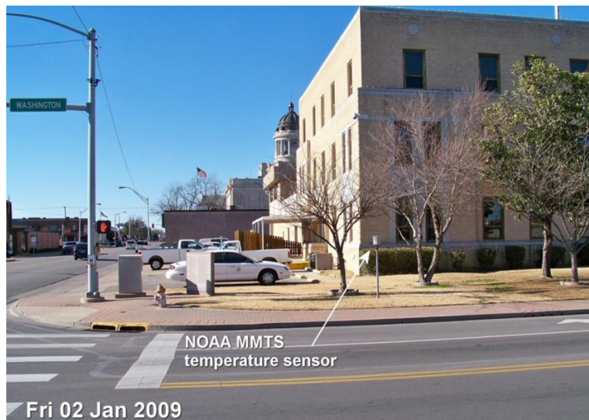
Figure 2 - USHCN Temperature sensor located on street corner in Ardmore, OK in full viewshed of multiple heatsinks.
